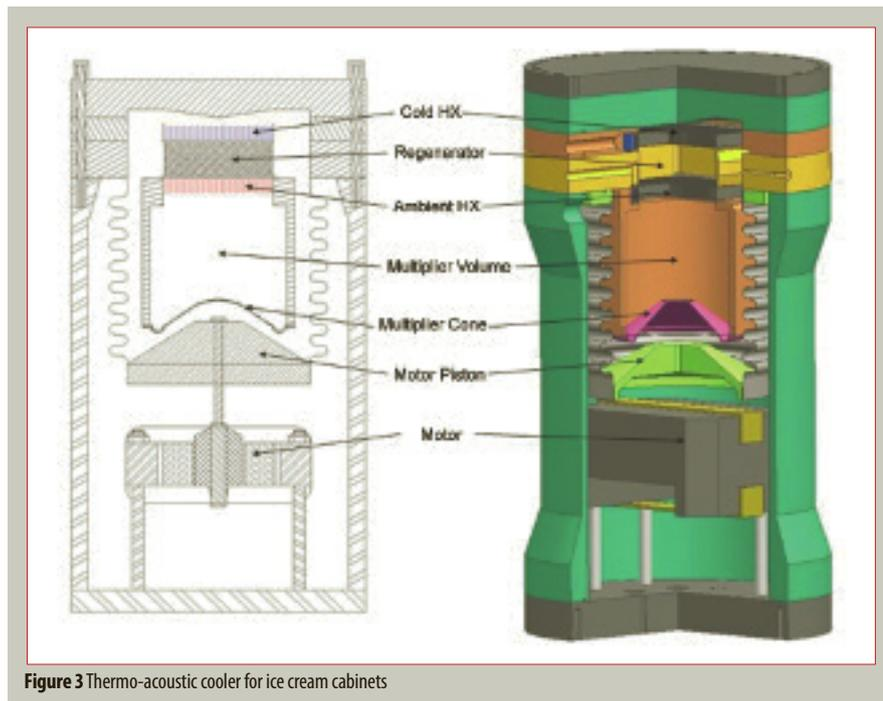
Figure 3 Thermo-acoustic cooler for ice cream cabinets
