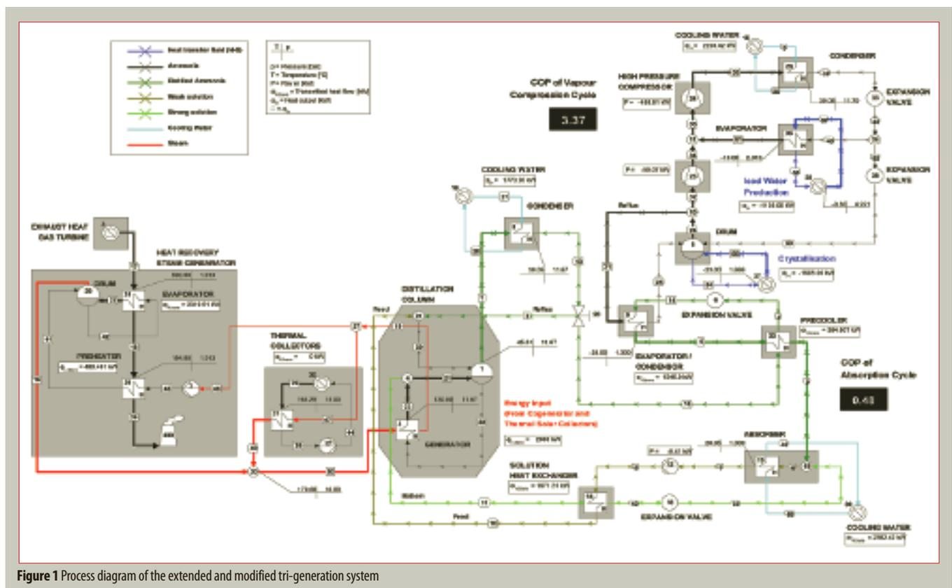
Figure 1 Process diagram of the extended and modified tri-generation system
